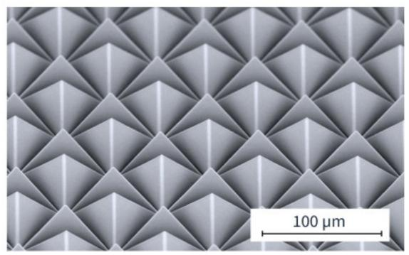
Retro-reflector: Fabrication of high-quality masters used in diverse replication technologies.
