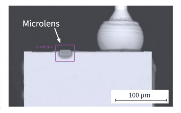
Microlens on EEL facet: Cylindrical microlens fabricated directly on the facet of a DFB laser to compensate the elliptical beam profile.
